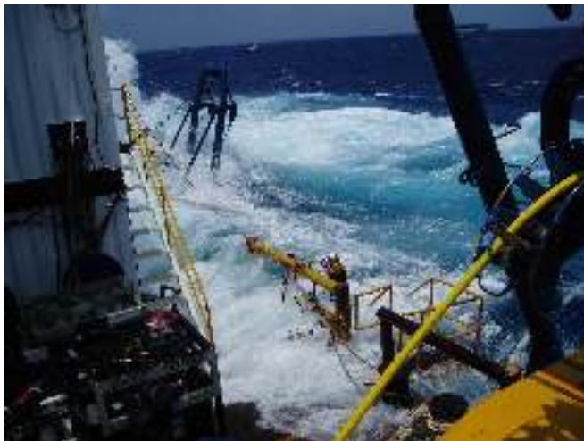
Figure: Wave has removed boat landing gear
