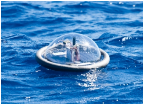
An ocean drifter, credit diydrones.com Diameter \approx 20cm, 1000s in the ocean
