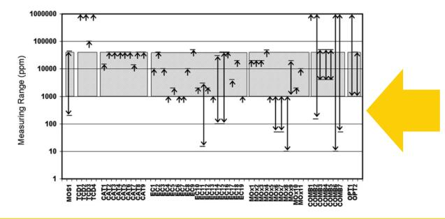
Measuring range of spot sensors<sup>6</sup> Most commercial spot sensors have LDL >=1000 ppm. Few have LDL = 10-100 ppm
