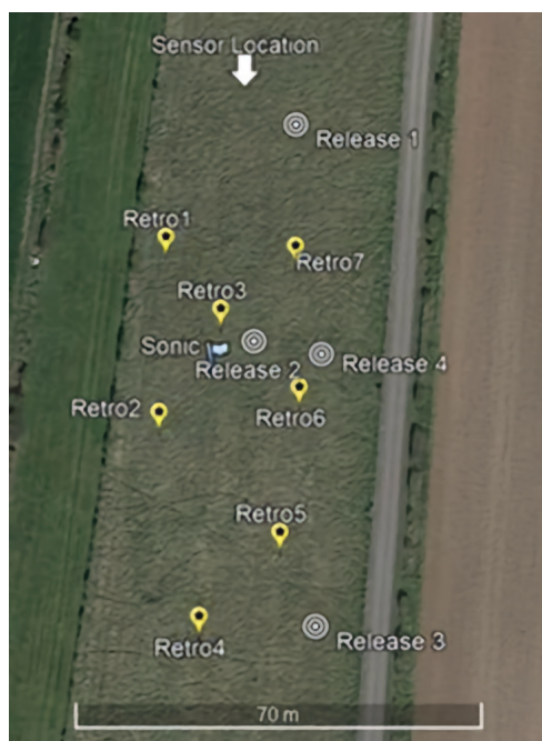
FIG 1. Methane release set up at the Chilbolton observatory, UK. Credit: Hirst et al. (2020) Supporting Information S1. A laser dispersion spectrometer measures path-averaged \text{CH}_4 concentrations between the sensor and each retros. "Sonic" indicates the emplacement of the 3-D ultrasonic anemometer measuring the wind speed and direction.
